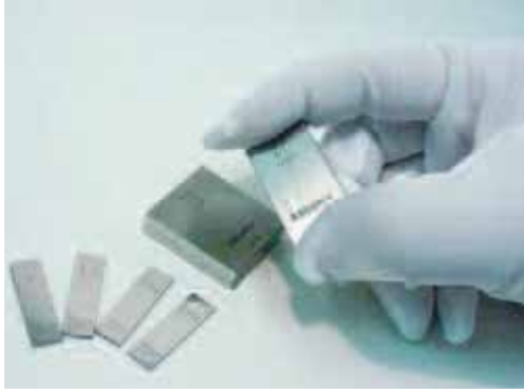
Fig. 2 Example gage blocks and use of white gloves
