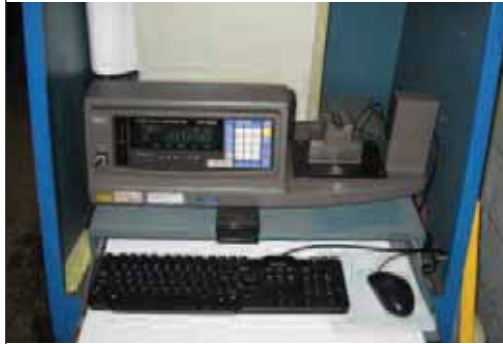
plating thickness inspection station with LSM-9506
